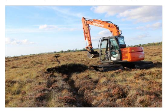
Figure 5.16 Machine currently used by Bord na Móna to block drains on the high bog (Hitachi Zaxis 70LC) © David Fallon (Bord na Móna)
